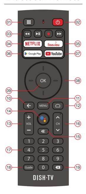
This Remote requires 2x AAA Batteries to operate. Insert the batteries, ensuring they correctly align with the polarity (+/-) markings found inside the battery compartment.
