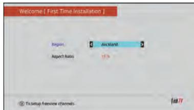
Note, in the First Time Installation, the STB will automatically install the Optus D1 Satellite Transponders. There is no need to perform LNB set-up, as LNB detection will be automatic. The STB will look for the preferred LNB settings and install the channels accordingly.
