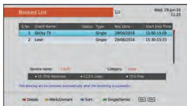
Note, this unit is a single tuner so this means there will be some limitations to what channels you can watch while recording. You will also be unable to book/record anything without first connecting a USB Device, as this unit is a USB PVR only and has no internal storage space.
