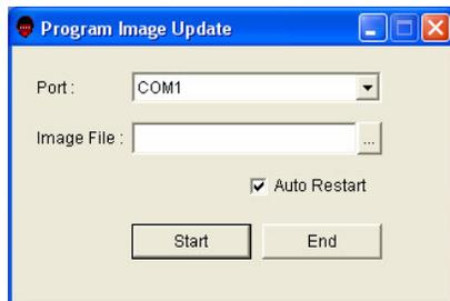
Select the connecting COM port, then select the firmware image file and press the Start button.
