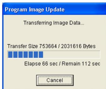
Turn on the receiver and the progress bar will update. The upgrade process will take approximately 5 minutes. The Receiver will automatically restart once the update process has completed. Do not turn the receiver off before the update process has completed.
