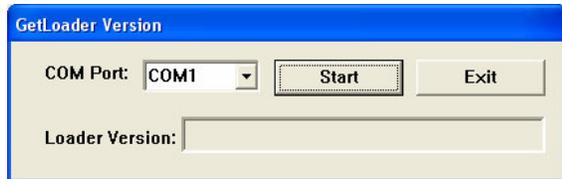
Press Start, and then turn on the Receiver. The loader version will display in the box.
