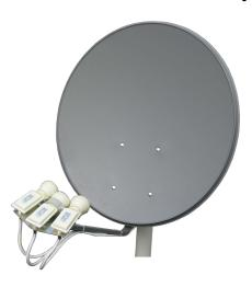
The Twin & Triple LNB plate has four holes and three slots. The middle slot is wider to allow two options for assembly. The plate can be used either on a 75cm or 90cm dish as a triple LNB system for the satellites Optus D1, Optus C1 & Optus D2. Or it can be used with two LNBs on a 60cm dish for Optus D1 & Optus D2.
