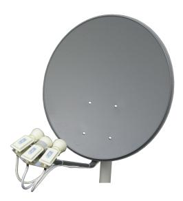
**Installation of the Twin system:** Align dish to D1 with meter on middle LNB. Remember that the LNB for Optus D1 is the LNB that mounts on the dish. The Optus D2 LNB is the one that hangs on the plate. Lock dish in place . Connect meter to the D2 LNB and adjust the skew of center LNB and plate for max signal for D2 . Remove the meter. Connect diseqc switch.
