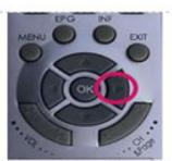
Now scroll down to LNB Freq2 using the down button. Then use the left and right buttons to change the LNB frequency.
