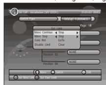
Figure 4. DiSEqC1.2 Motor Limitation
